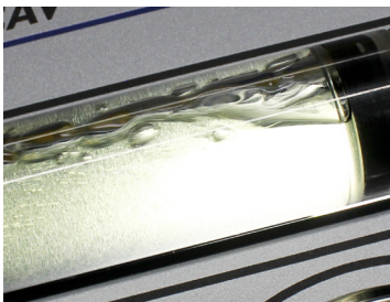
Demonstrate Laminar Flow - Occurs when air enters the oil flow
