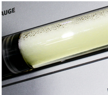
Demonstrate cavitation and pseudo-cavitation - Occurs when inlet is restricted or when there is an air leak present
